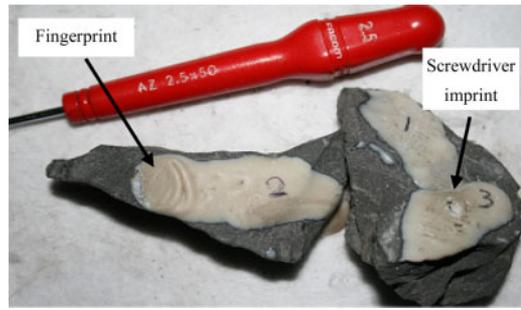
Figure 10. Glue aspect after 16 h curing (12°C) and heating under a spotlight (~60°C) during a few seconds. The glue softens so it can be easily moved with a finger or a screwdriver.
