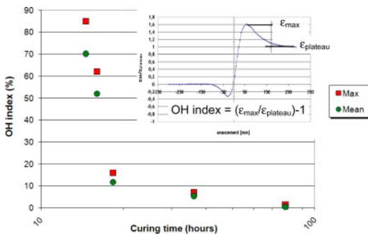
Figure 3. Curing time impact on the “overcoring hump” as quantified by the OH index.
