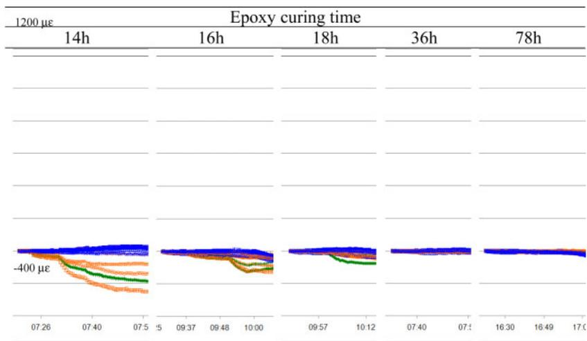
Figure 5. Curing time impact on the initial jump in strain readings at the onset of flushing. From left to right are shown the strain responses of the CSIRO Hi cells to the onset of flushing for increasing curing times (tests TC33, TC32, TC31, TC35, TC36 respectively). For comparison, all graphs have the same y-axis scale range.
