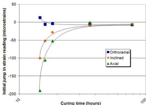
Figure 6. Curing time impact on the initial jump in strain reading at the onset of flushing. Each point corresponds to an average for all gauges of the same orientation.
