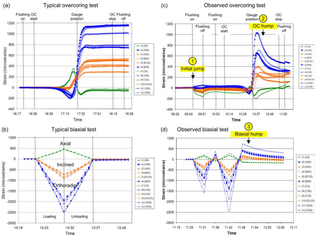
Figure 1. Left: Typical evolution curves for strains at the vicinity of a pilot hole (a) during an overcoring test and (b) during a biaxial test. Right: Strain curves recorded in Tournemire 2005–2006 experiment (c) during an overcoring test and (d) during a biaxial test.
