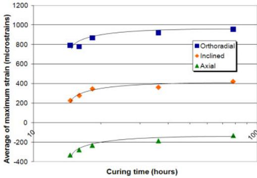
Figure 8. Curing time impact on the average amplitude of peak strains that develop during overcoring. Each point represents average value for all gauges of the same orientation.
