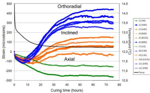
Figure 9. Typical evolution of strains and temperature recorded in Tournemire tests during glue hardening (test TC36).
