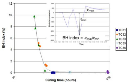
Figure 4. Curing time impact on the “biaxial hump” as quantified by the BH index.
