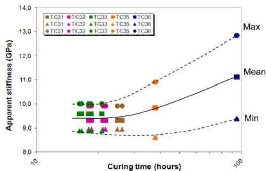
Figure 7. Curing time impact on the apparent stiffness of overcored samples determined from biaxial test.
